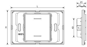
Mounting with frame: 122 x 77 (L x H) Mounting without frame ('NF): 120 x 80 (L x H)
