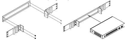
**3** Secure the rack bracket or faceplate bracket assembly to the switch.
