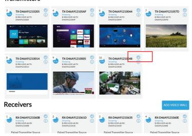
The discovery process will identify all transmitters and receivers on the system and displays. Devices will be discovered and assigned a transmitter or receiver number. Transmitter and receiver numbers will correlate directly with the inputs or outputs respectively for control system integration, similar to traditional matrix switchers.
