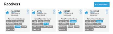
Record the Receiver number, MAC address, and connected display type/location for use during control system integration.
