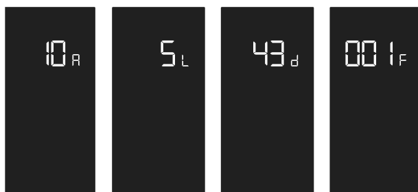
Example of displaying the physical address 10.5.43 (device nr. 43, installed on the line 5 of the area 10) and the firmware release 001
